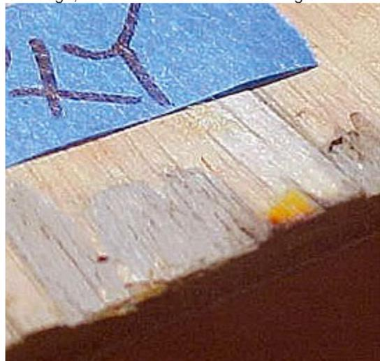
If a piece of veneer is chipped off on the edge of a board we'll glue in a new piece. I'll find a teak remnant in the shop that matches the color and texture of the missing veneer, trim and shape it to fit, epoxy it in, then sand it all fair. Again, in the end it may show a little, but should look far better than leaving it chipped. Fill, fix and fair whatever you feel will add to the overall restoration before moving to the finishing steps.
